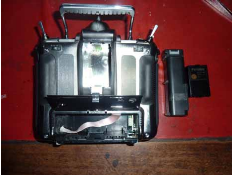
Figure 54 Stage 1 Complete - Module and Battery Removed
