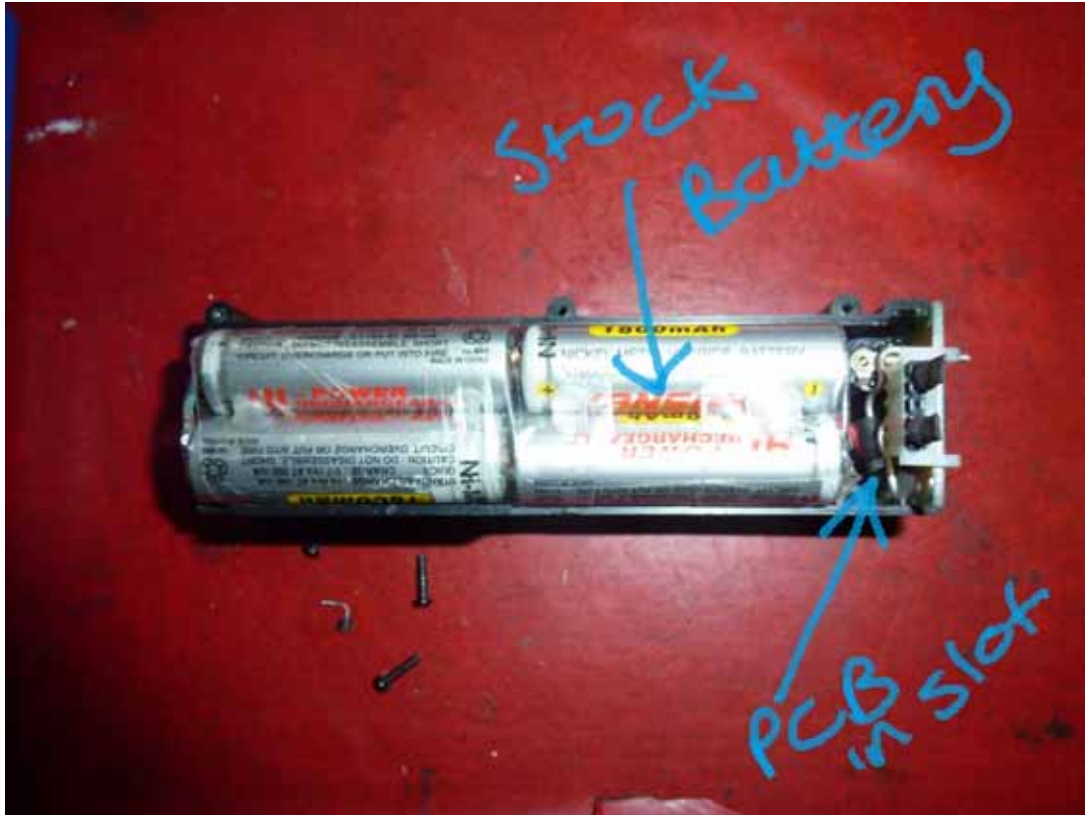
Figure 48 9Z Transmitter Battery Disassembly
