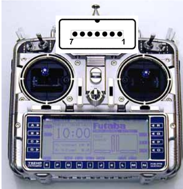
Figure 81 CAMPAC Pin-Out (Note: Reversed pin numbering)
