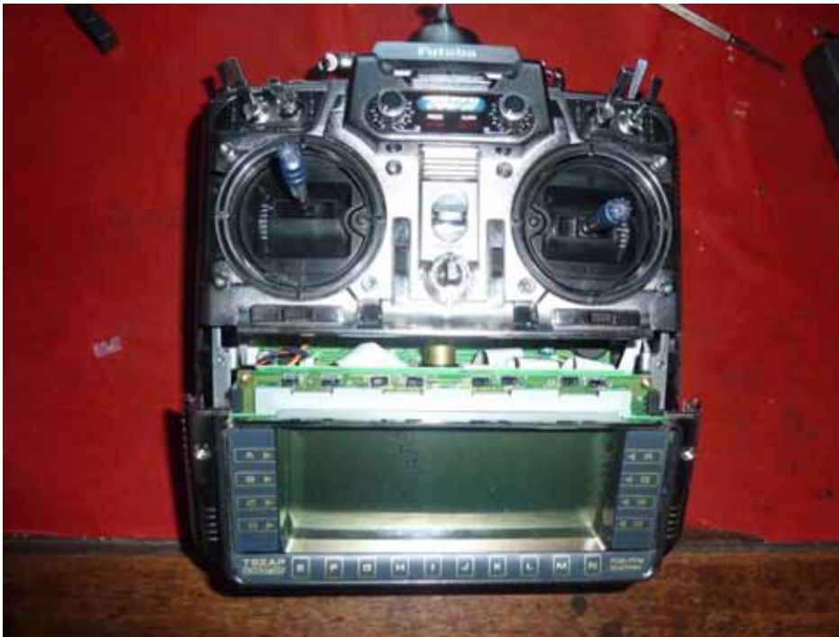
Figure 71 LCD Panel now completely removed (retaining plate/lugs on top)
