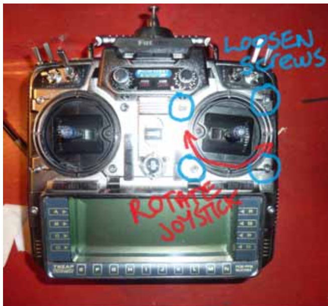
Figure 34 Changing the Rotational Position of Joysticks
