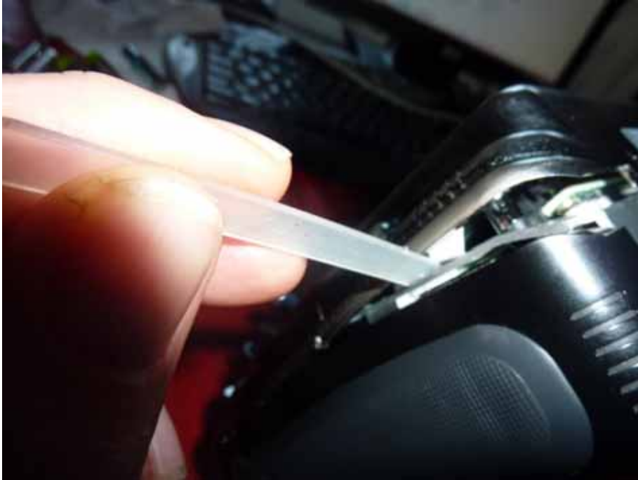
Figure 74 Cables at sides of LCD Panel that get trapped
