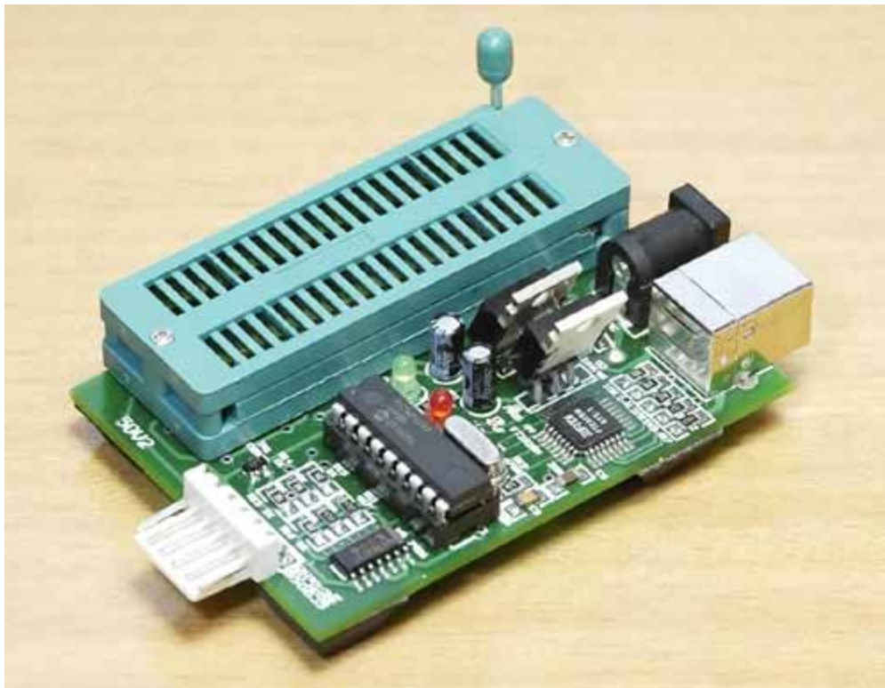
Figure 8 USB ICP PIC programmer with ZIF 'hook up' for the chip in green/blue.
