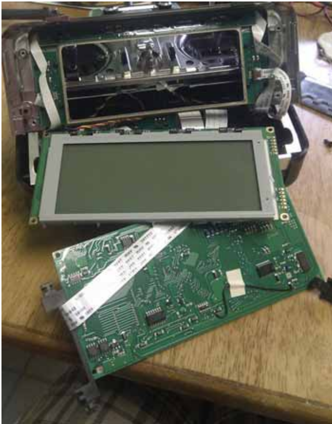
Figure 28 LCD Assembly removed and partially disassembled
