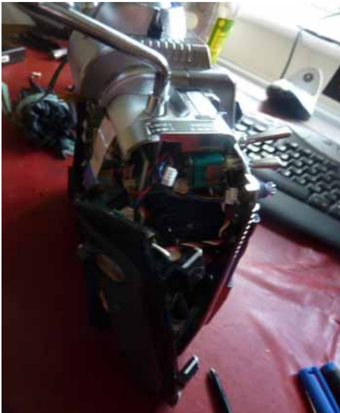
Figure 65 Case sides slid outwards and removed
