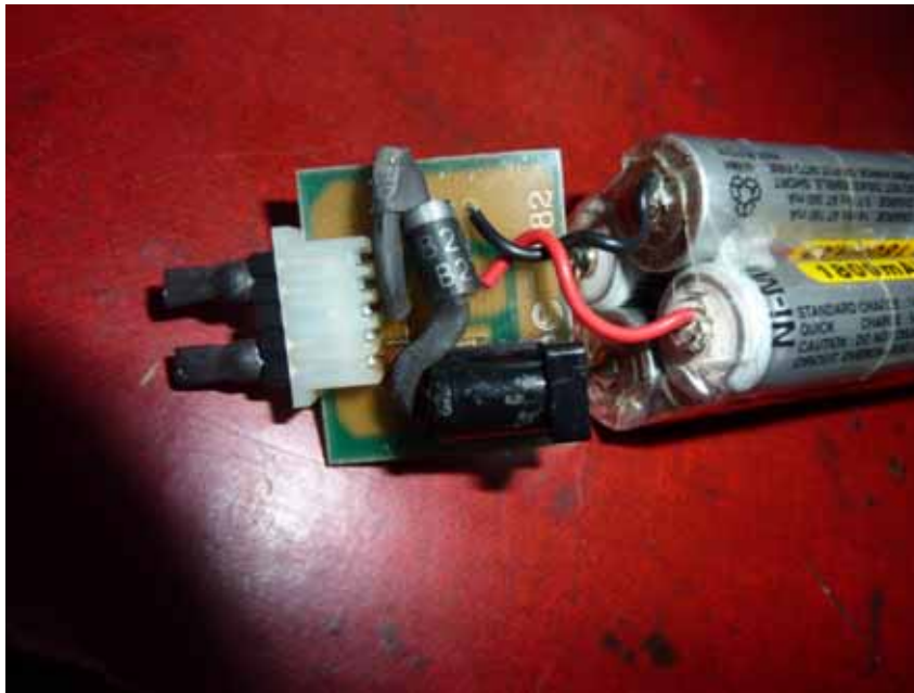
Figure 50 New 3A diode soldered to PCB (Note: Silver line on diode indicating orientation)
