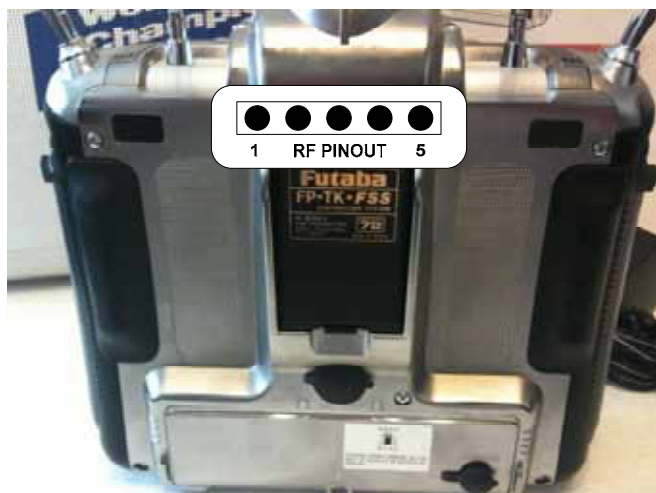
Figure 79 Futaba RF Module Pin-out Numbering
