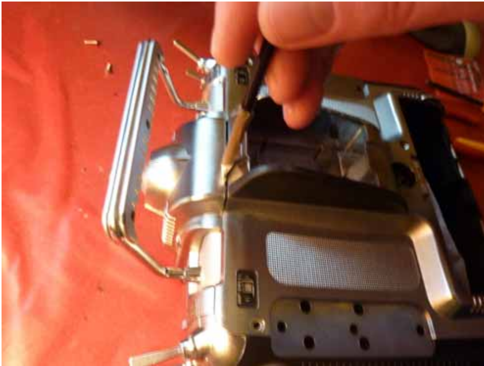
Figure 61 Protect a screwdriver and lever case top up to refit case back
