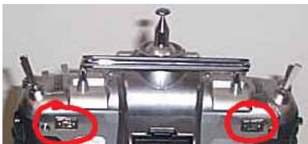
Figure 1 The 9ZA's 'Snap Roll' switches, that are missing in the 9ZH version
