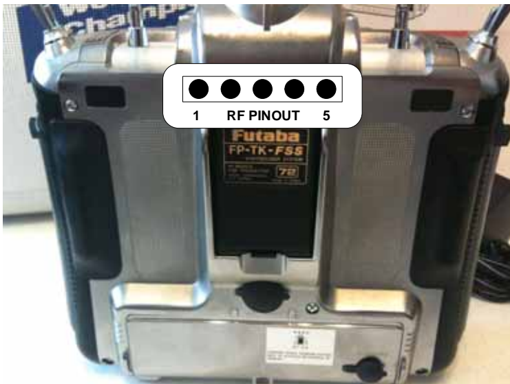
Figure 31 Futaba RF Module Pin-out Numbering
