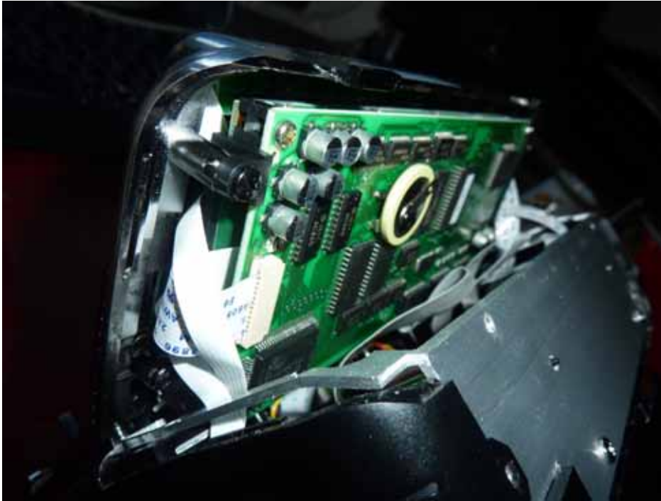
Figure 70 Lever up PCB panel
