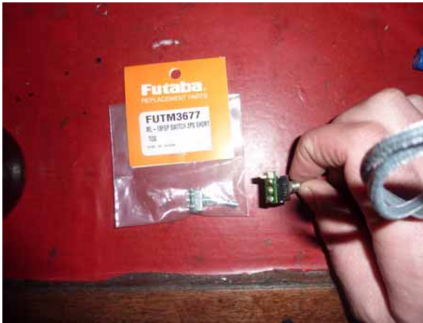
Figure 9 Corner Switch Replacement - NOTE: 8U SWITCH PART NO. IS SHOWN!
