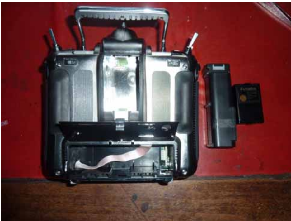
Figure 62 Refit battery hatch
