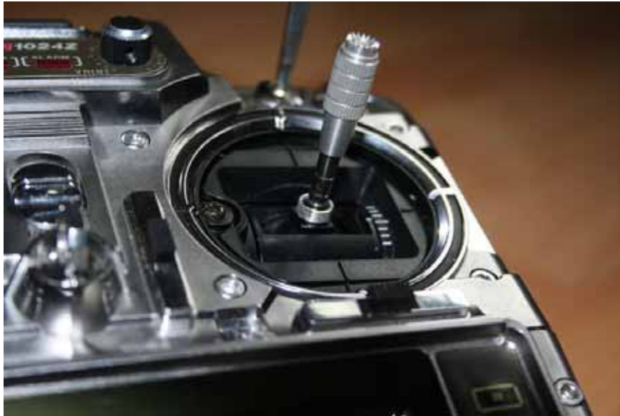
Figure 36 Metal joystick strengthening collet
