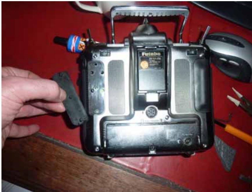
Figure 55 Removing the comfort grips
