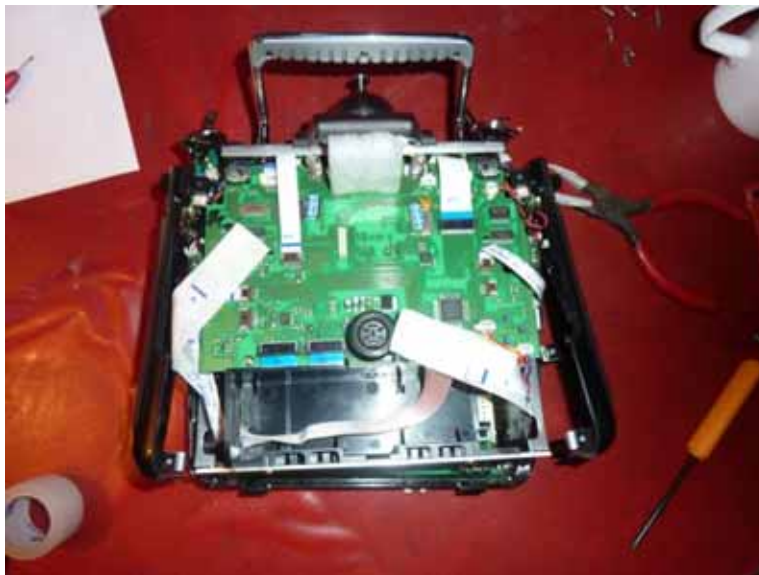
Figure 73 Ribbon cables with masking tape fed back through case
