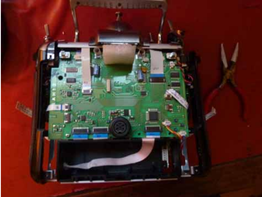
Figure 67 - Partial Step 3 Disassembly Option
