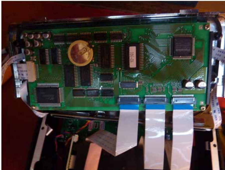
Figure 72 LCD Panel flipped over backwards for access
