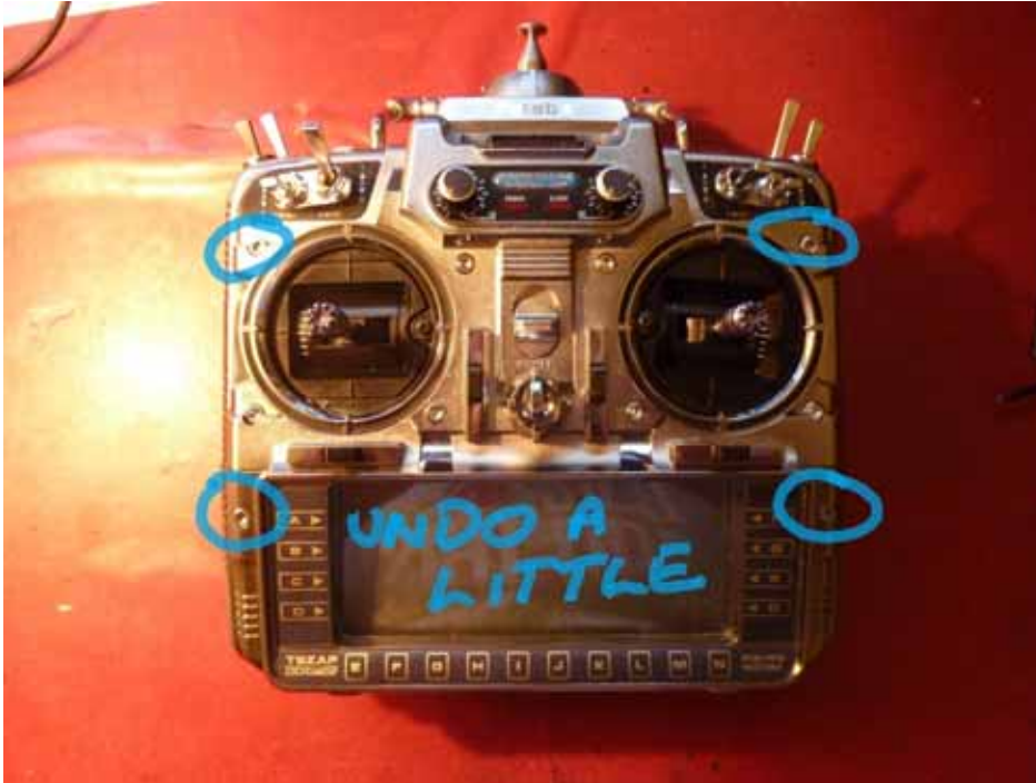
Figure 60 Screws to loosen to allow play in case sides
