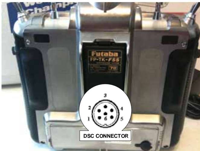
Figure 80 DSC/Trainer Port Pin-out (6 pin DIN)
