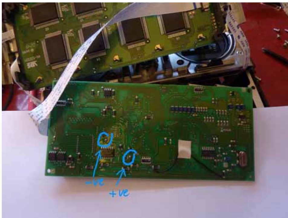
Figure 26 Top PCB 'Flipped' and Battery Terminals Exposed
