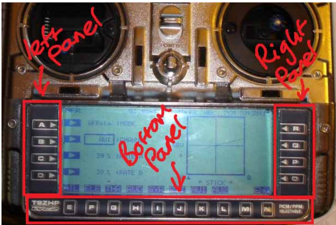
Figure 21 The three LCD Button Panels shown on a 9ZHP WC2
