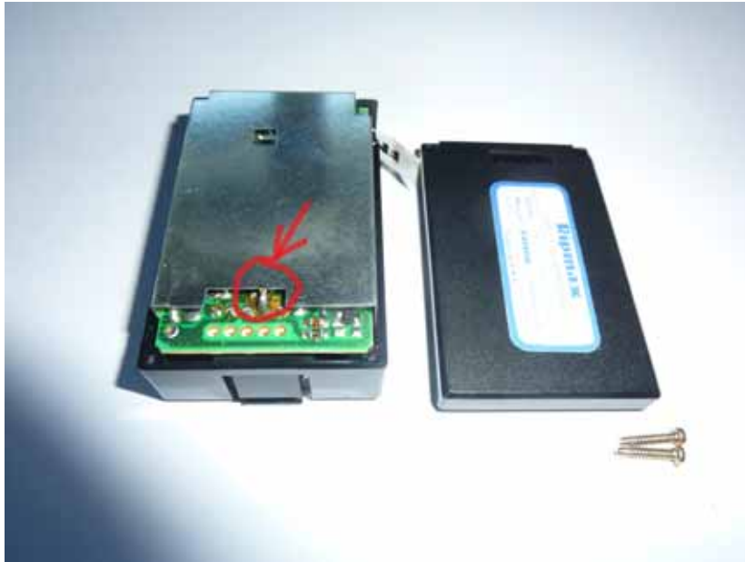
Figure 32 Weak solder joint in RF Module
