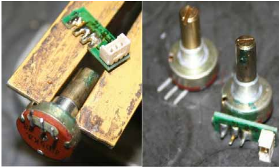
Figure 20 Desolder the connector PCB (green) from the POT
