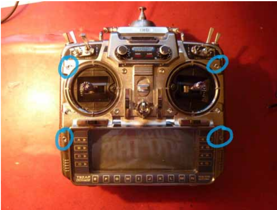
Figure 63 Allen key screws to remove
