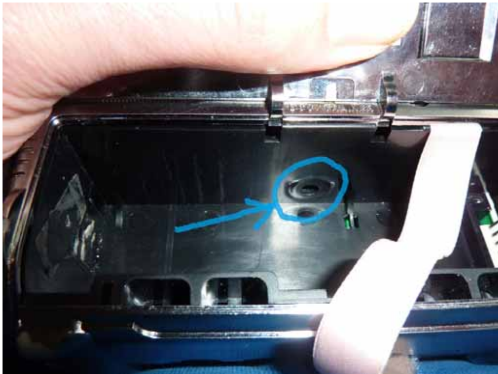
Figure 23 The access hole for the aerial retaining bolt in the battery compartment
